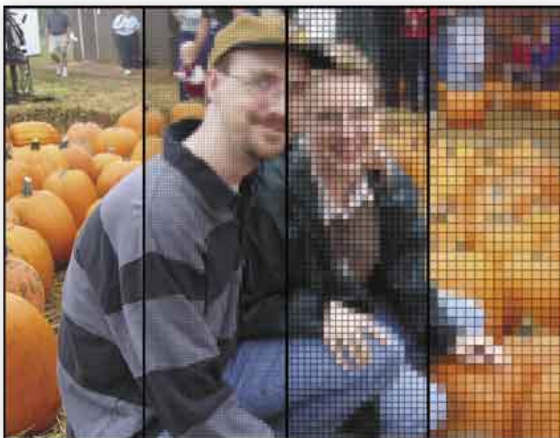
Figure 2. The more pixels, the smoother the photo. The left part of the photo is the smoothest; it has the most pixels in it. As the pixel count decreases left to right, the quality also decreases.
